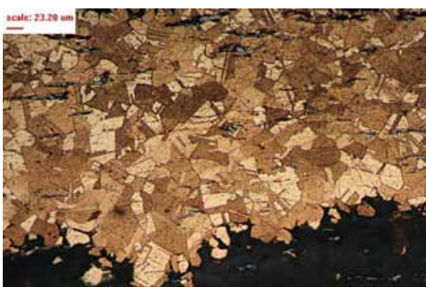
Fig. 4: Pin, Sg76-5. Left: Longitudinal section, OM image of the etched sample showing recrystallized twin grain structure with blue-grey elongated sulfide inclusions. Right: Full fragment. (Etchant: aqueous ferric chloride)
