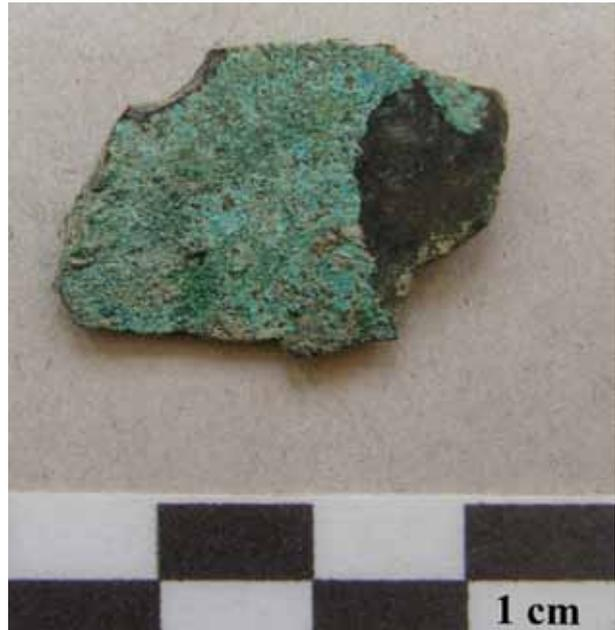
**Fig. 5:** Sheet fragment, Sg76-10. **Left:** Longitudinal section, OM image of the etched sample showing recrystallized twin grain structure with blue-grey elongated sulfide inclusions. **Right:** Full fragment. (Etchant: aqueous ferric chloride)
