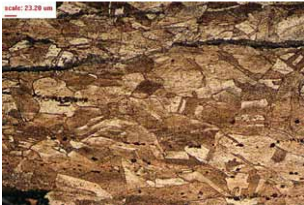
Fig. 7: Pin, Sg76-7. Left: Longitudinal section, OM image of the etched sample showing worked deformed grains and distorted twin bands. Right: Full fragment. (Etchant: aqueous ferric chloride)
