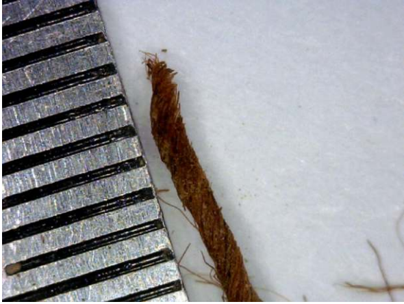
Fig. 6: Photomicrograph of thread made of vegetal fiber, Z-spun.
