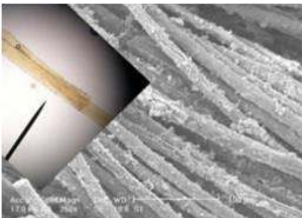
Fig. 8: Scanning Electron Micrograph of vegetal fibers (x250).
